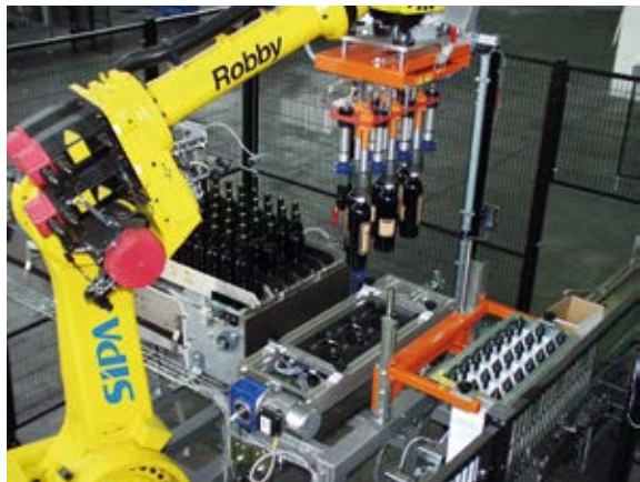
Multiple gripping head (pneumatic membrane gripping heads and suckers) and vertical tilt unit for cartoning flipped bottles
