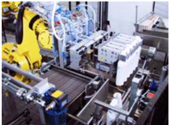
Versatile gripper with pincer and suction cups for horizontal cartoning of paper-wrapped bottles, handling both products and cardboard dividers.
