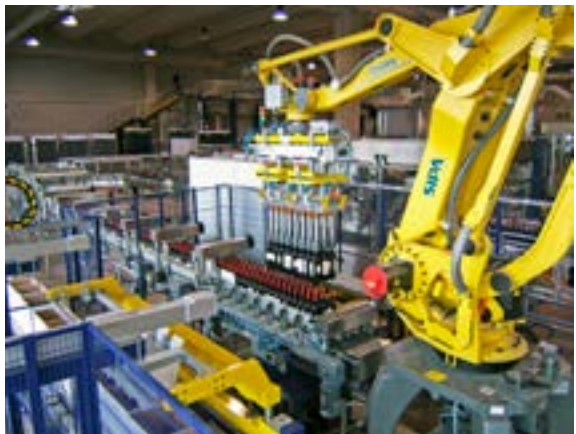
Combined cartoning solution for flat and vertical bottles with interlayer pads inserting device Multiple gripping head (pneumatic membrane gripping heads and suckers) and vertical tilt unit for cartoning flipped bottles
