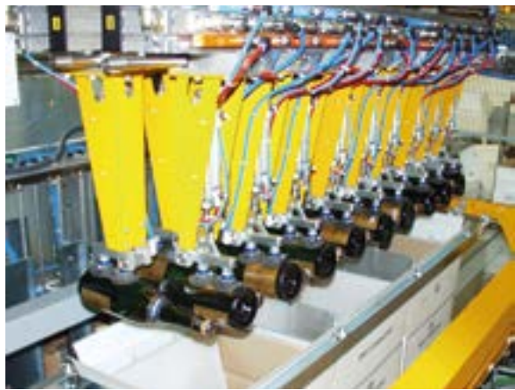
Sucker pick-up head for cartoning flat and crossed bottles
